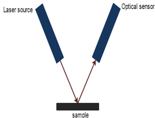
Figure 2, the trigonometric method
