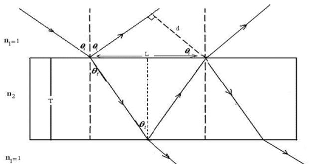
Figure 6 the optical path beams output from multiple reflections in the glass
