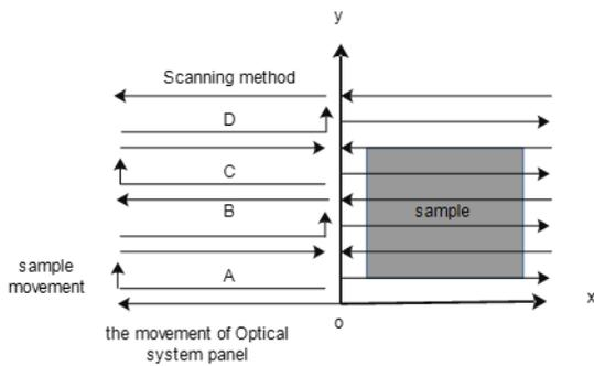
Figure 3, the laser scanning method
