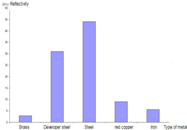
Figure 4 the disparity in the amount of reflectivity between metals listed in the table 1.
